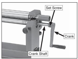
Figure 8. Crank mounting.
